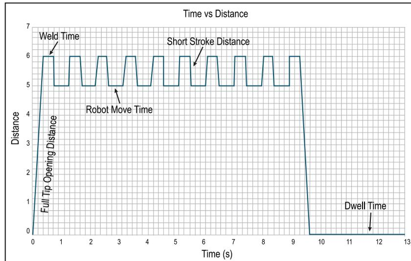
*The motion profiles of real-world automobile manufacturing robotics like weld guns are much more complex than a simple open-and-close press cycle.*
