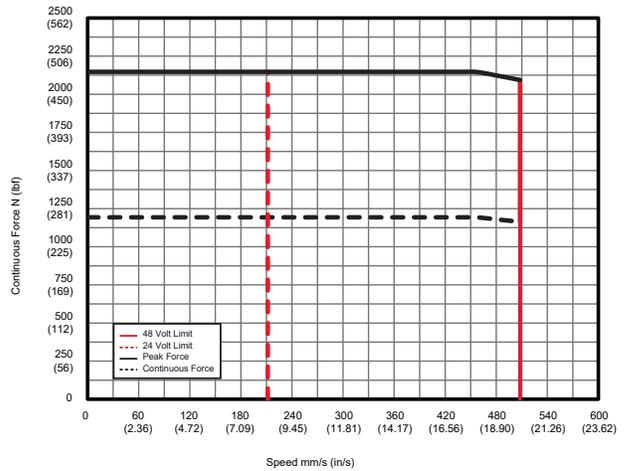
\*Test data derived using NEMA recommended aluminum heatsink 10" x 10" x 3/8" at 25 °C ambient.
