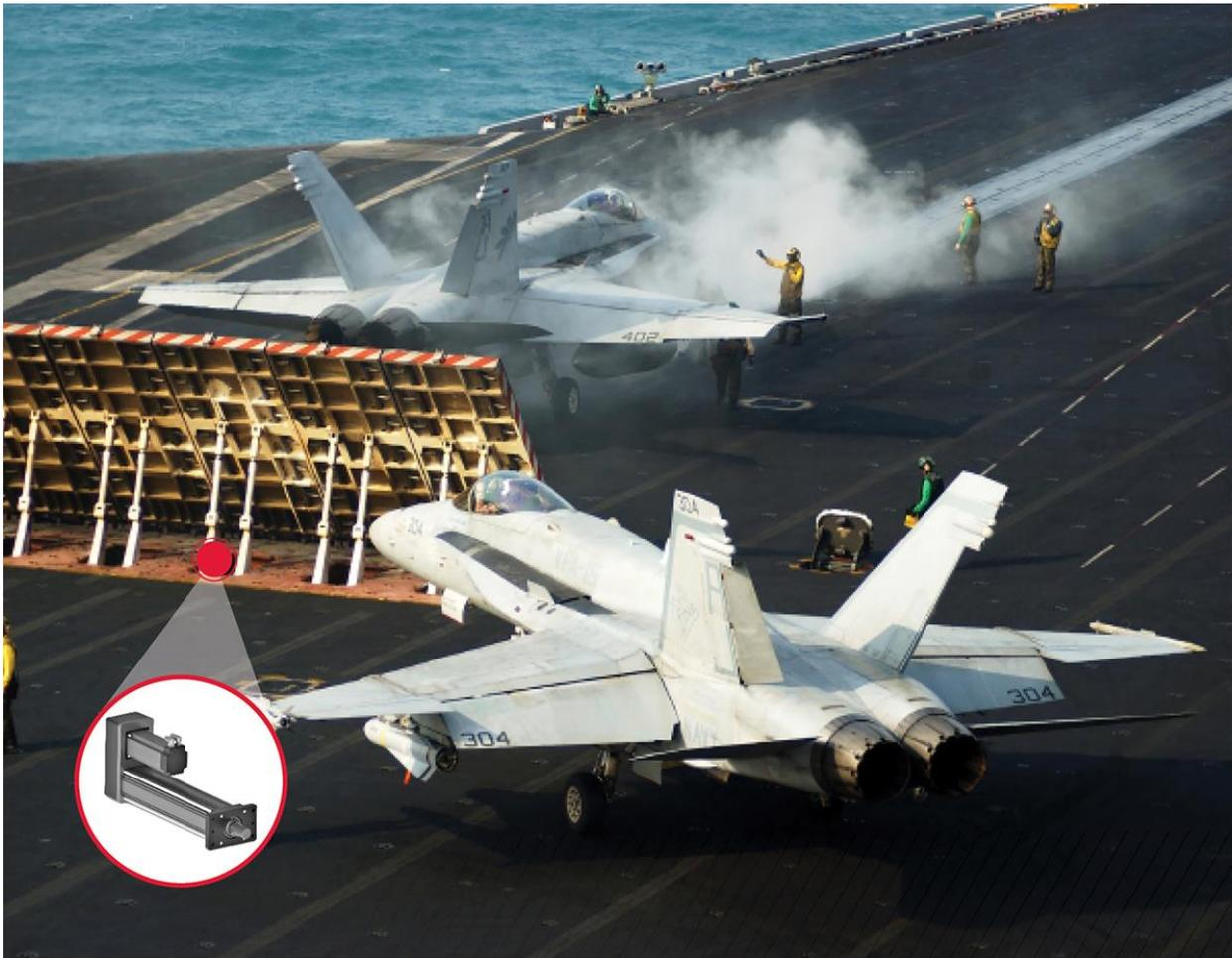
Figure 4 - A jet blast deflector is raised to protect one F/A-18 Hornet from the jet exhaust of another.
