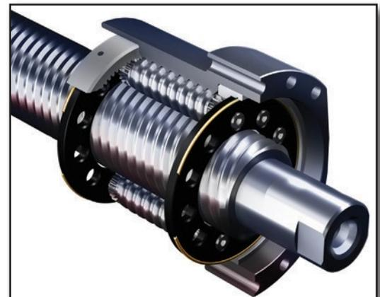
pal to ball screws, with a nut running along a threaded rod. Unlike the balls in a ball screw, roller screw nuts utilize threaded rollers that are geared with respect to each other and the nut housing much like a planetary gearbox.
