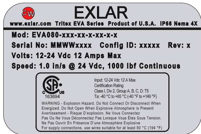
Figure 1 - Typical Label Specifications
