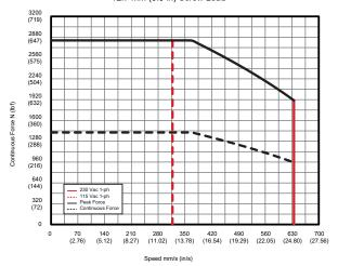
\*Test data derived using NEMA recommended aluminum heatsink 10" x 10" x 3/8" at 25 °C ambient.
